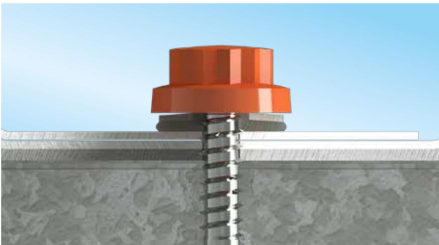
**An effective seal does NOT mean flattening the washer**
